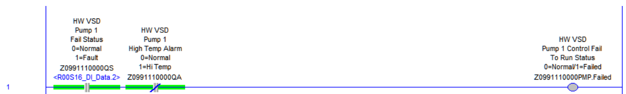
Figure 7-9 Sample Alarm Cascading Interlock
